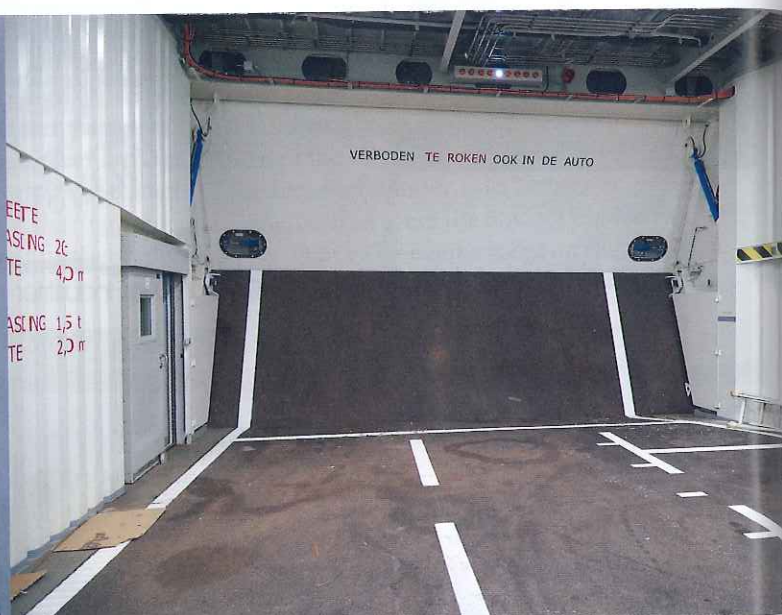
Weather permitting, the upper part of the two-piece access doors can be opened for ventilation purposes during the crossing.
