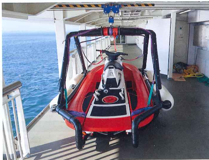
The MOB boat comes in the form of a water scooter that is launched from the bicycle deck - Deck 4.
