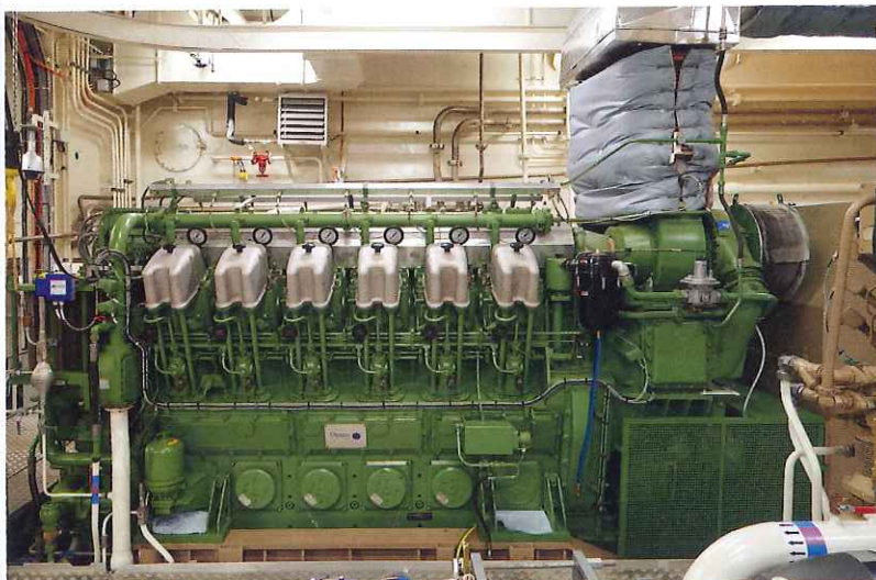
The two single fuel (diesel) engines are similar to the dual-fuel ones and have been installed for redundancy's sake. All four engines drive generators that provide electrical power to the four Rolls-Royce azimuth thrusters.
