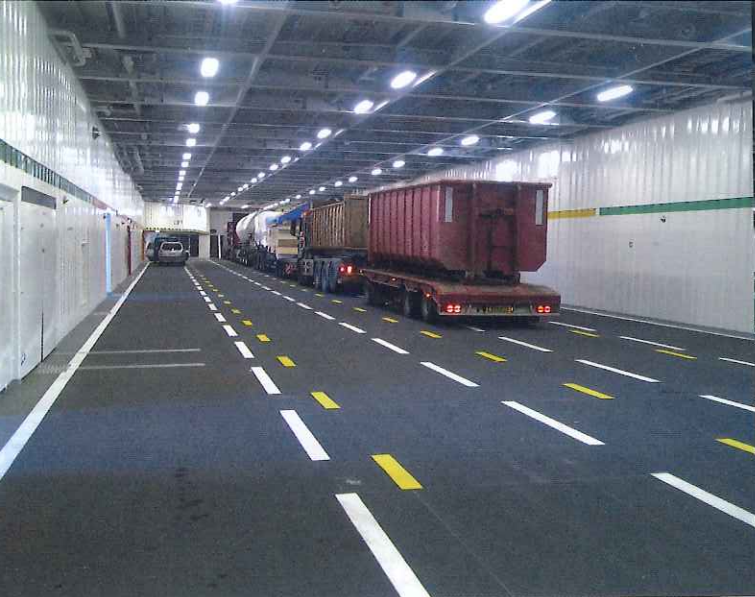
The main vehicle deck's full-height central part between the engine casings with colour coded stairs has four truck lanes or alternatively five lanes for cars.
