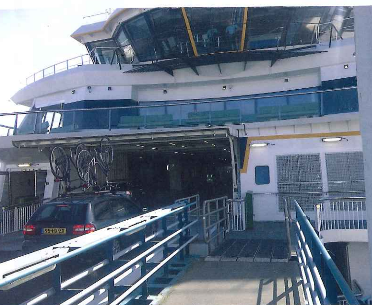
To connect with the existing linkspans, the access doors on the main and upper level are offset to the ship's Wadden Sea side.
