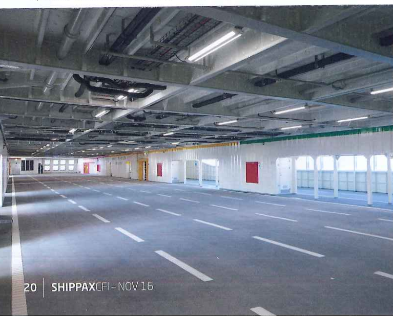
The upper car deck can accommodate 209 cars. On a clear day, it gets plenty of natural daylight through large windows, largely replacing more expensive artificial lighting.
