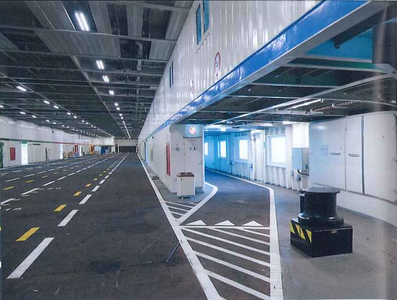
The outer car lanes on the main vehicle deck (one on either side of the casings) have a height of 2.6m with the upper level being occupied by the semi-open bicycle deck.
