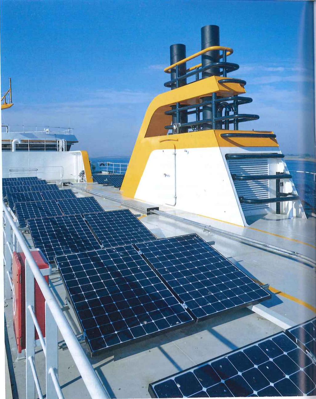
TEXELSTROOM boasts 462 solar panels - equivalent to 700 m 2 - the energy of which is stored in batteries.
